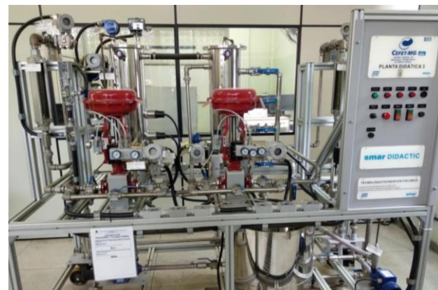
Foundation Fieldbus Didactic Plant
